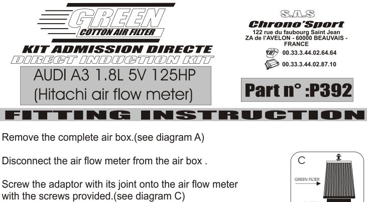
Fix the filter with the attaching bracket provided onto the original air box fixing.(see diagram B).
